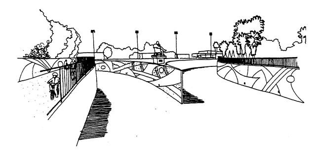
In the area between the Sepulveda Basin and Universal City, the river was channelized in the late 1940s and early 1950s. The right-of-way here varies in width from 120 feet to 250 feet. A 38-foot wide strip runs along the north side of the channel and at times on the south side as well.
